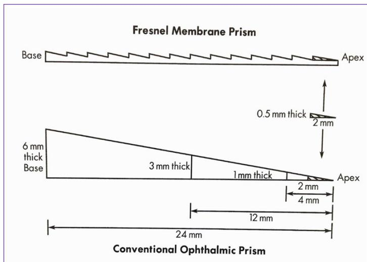
**Figure 1.** Fresnel membrane prism compared to conventional ophthalmic prism.<sup>7</sup> Reprinted with permission. Retrieved from [www.fresnel-prism.com](http://www.fresnel-prism.com).
