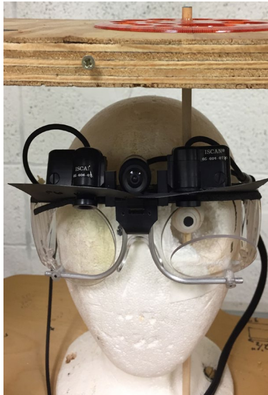
Figure 6. Apparatus used to measure the noise in the ISCAN eye-tracker at various angles of artificial eye rotation.
